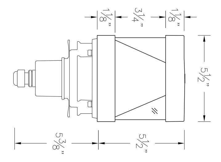
99 852 Shown on Bollard Tube 99 614 (SCALE 1:2)
