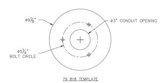
Figure 1: Anchorage Template
