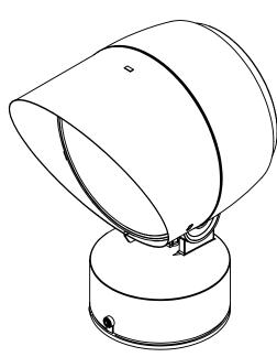
84208 SHOWN WITH ELLIPTICAL SPREAD LENS ACCESSORY 71120 LENS IS ROTATABLE 360°
