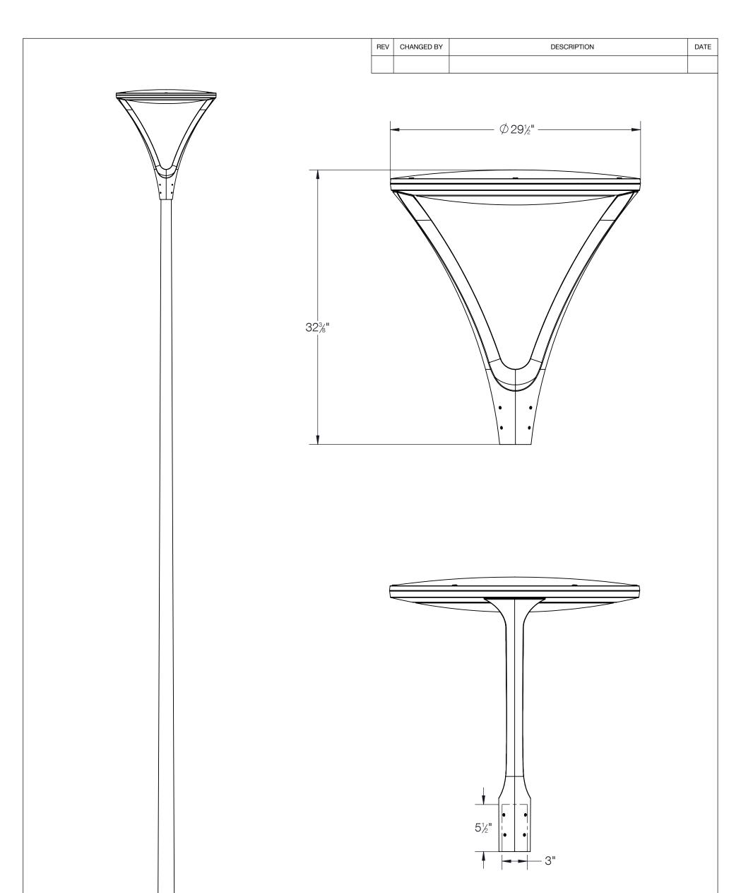
NOTE: TENON OR POLE INSERTION DEPTH OF 5-1/2" REQUIRED FOR PROPER INSTALLATION
