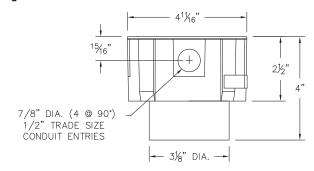
SMALL OPENING WIRING BOX DETAIL
