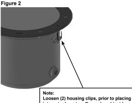
into outer housing. Once placed inside outer housing, tighen clips until secure.
