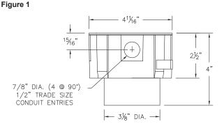
SMALL OPENING WIRING BOX DETAIL
