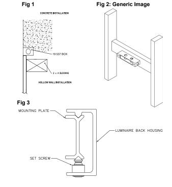
SECTION VIEW: MOUNTING DETAIL (NOT TO SCALE)
